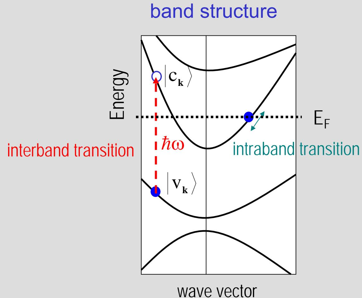
$$\underline{\text{Im}\epsilon_{\alpha\beta}(\omega)} = \frac{4\pi e^2}{m^2\omega^2} \sum_{c,v} \int d\mathbf{k} \langle c_{\mathbf{k}} | p^{\alpha} | v_{\mathbf{k}} \rangle \langle v_{\mathbf{k}} | p^{\beta} | c_{\mathbf{k}} \rangle \delta(\varepsilon_{c_{\mathbf{k}}} - \varepsilon_{v_{\mathbf{k}}} - \omega)$$
